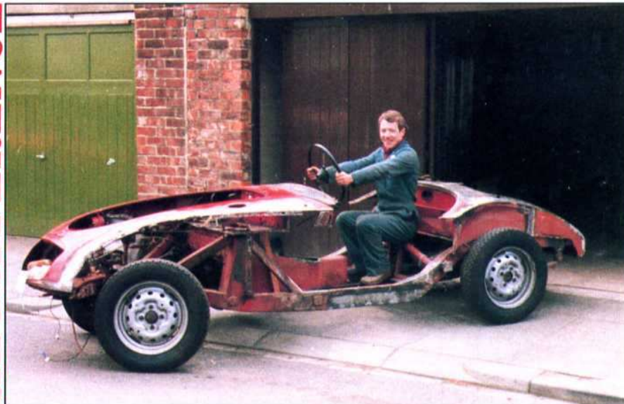
Above left, the restoration involved stripping the car down to a rolling chassis and removing and overhauling all mechanical parts Above right, thorough preparation at this stage is vital for a successful restoration — here the body seams are filled and sealed
