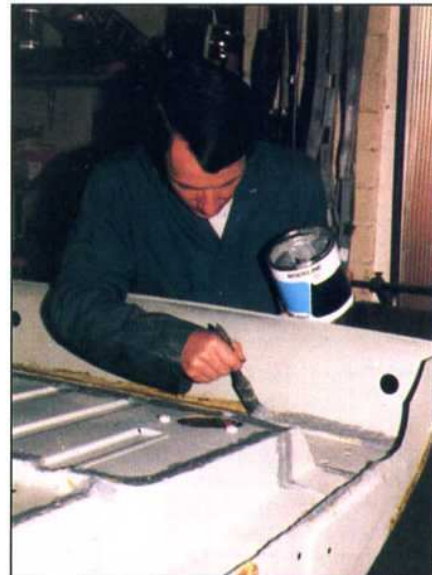
Above left, the restoration involved stripping the car down to a rolling chassis and removing and overhauling all mechanical parts Above right, thorough preparation at this stage is vital for a successful restoration — here the body seams are filled and sealed
