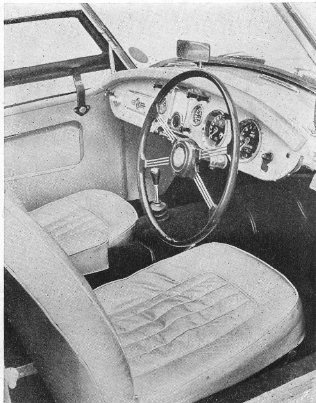
Cockpit layout is unchanged from the normal M.G. A., but the seats are more heavily padded and better shaped, while the instrument panel is covered in leather.
