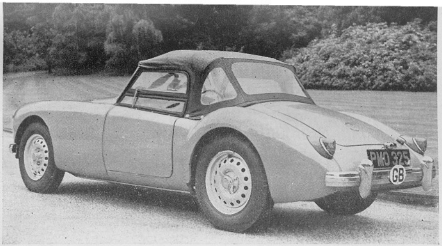
The hood, although rather cumbersome to erect, is extremely efficient in keeping out rain and draughts. Centre-lock pressed steel wheels are standard equipment.
