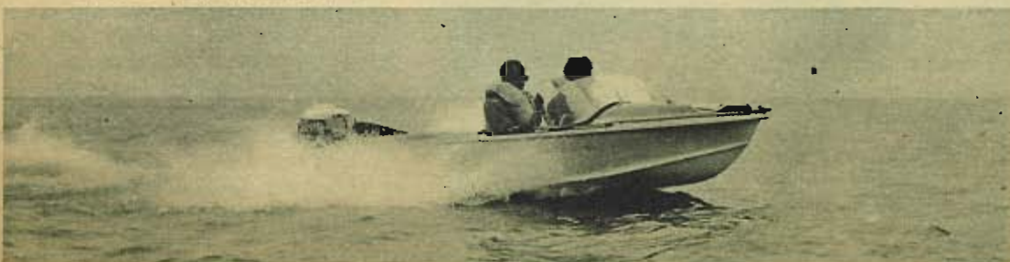
The 18 h.p. British Anzani Magnatwin is a two-stroke outboard motor with electric starting. The engine is shown above, and below, the picture shows the engine pushing a 14-foot fast runabout across the Channel.
