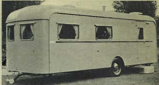
(Right) PILOT PANTHER Mk. X. This 4-berth caravan has increased height, giving 7 ft. headroom throughout. It has grey Hornitex on the walls and ceiling of the kitchen, and bird's-eye maple Hornitex on the ceiling of the lounge. There is a built-in television, a refrigerator, and a 5 ft. bath in the bathroom. The caravan is 22 ft. long. Price £1,245.
