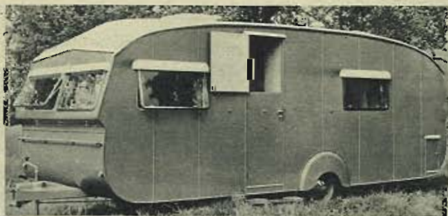
(Left) JUBILEE 'MAY-FLY'. 22 ft. long and 7 ft. 6 in. wide, this caravan weighs 35 cwt. It is fitted with 2 single beds and a double bed, a separate end kitchen and toilet compartment. All furniture is oak finished and hand-polished. The outside is panelled in aluminium, and the inside in plywood, with fibreglass insulation. Price £675.
