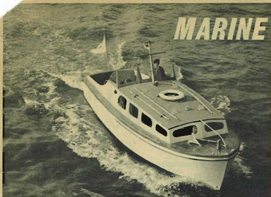
The Thornycroft 28 ft. 6 ins. "Danielle" class glass fibre cabin cruiser is powered by a Thornycroft 30 h.p. diesel engine giving a speed of 9½ m.p.h. A boat of similar design, but with twin petrol engines each of 20 h.p., and an alternative accommodation arrangement, can be seen at the Motor Show.
