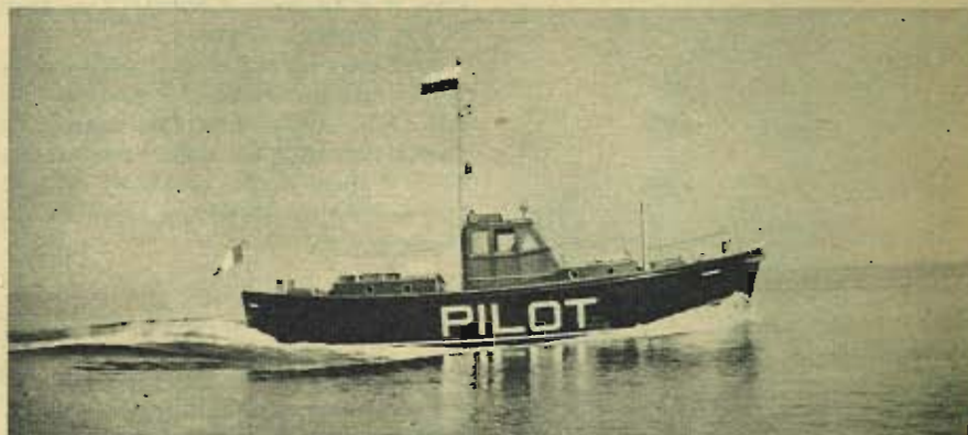
(Above): An Irish pilot vessel powered by Gardner 4LW engine developing 56 h.p. at 1,300 r.p.m. The Gardner 4LW marine propulsion diesel engine is shown below. It has direct driver reverse gear developing 56 h.p. at 1,300 r.p.m. for continuous heavy duty; 62 h.p. at 1,500 r.p.m. for yachts, cruisers, etc.; 71 h.p. at 1,700 r.p.m. for high speed craft.
