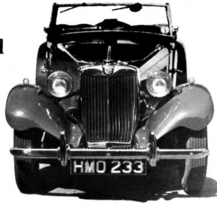
Still undisguised, the radiator has changed little since the days of the first series M Midgets; the flat, octagonal filler cap is functional, not just ornamental.
