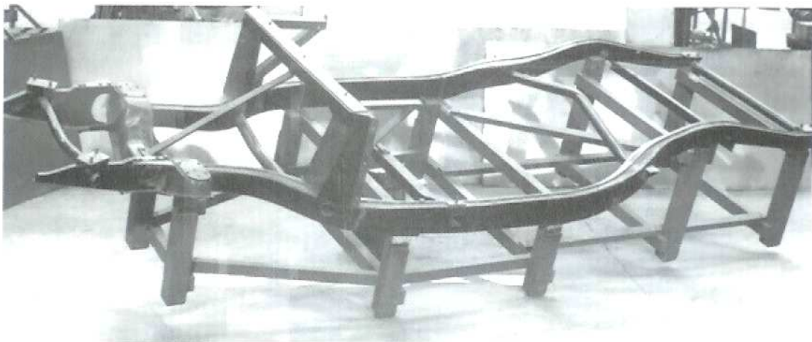
Chassis Jig for CKD frame construction
